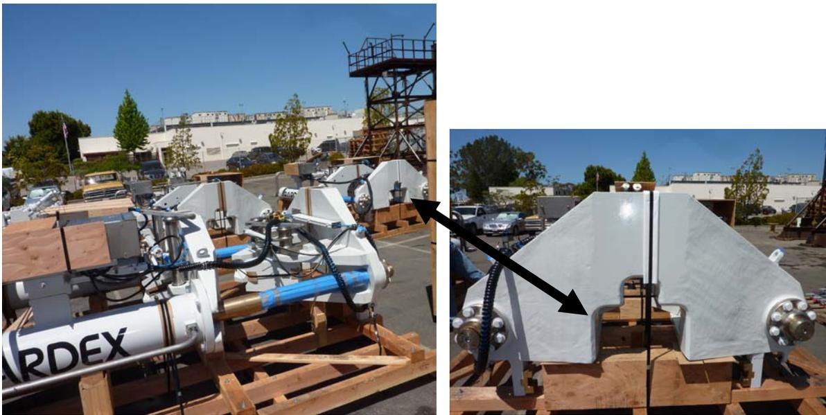
*Moveable chain jacks Note keyhole (cut-out) in lower arm for chain to pass through.*
