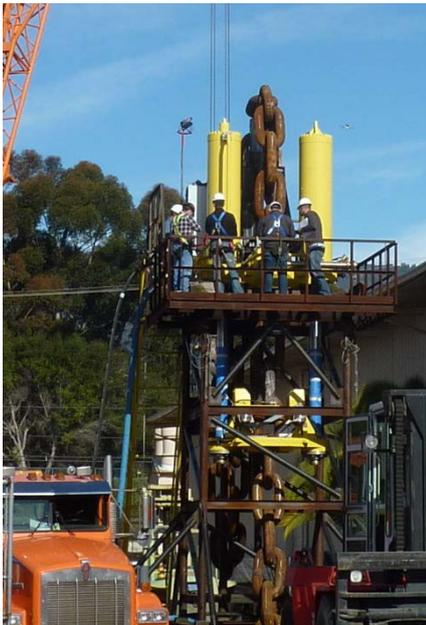
In the photo at left, Bardex engineers are preparing a test. Note the size of the 165mm chain as it rises through the travelling crossarm and latches at bottom, passes through the fixed crossarm and latches and on exit from the chain jack, drapes over the turndown sheave.
