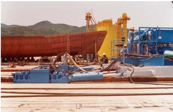
Of course Bardex is renowned globally for its skidding systems and over the last 45 years we have supplied many gripper jack skidding systems to yards worldwide for ship extrusion, load and recovery, and transfer applications generally for vessels, modules and offshore structures. Our recent order for a LORS (Load out and recovery system) is for handling vessels and offshore structures of up to 13,000 tonnes but Bardex has supplied systems for skidding ships up to 24,000 tons.
