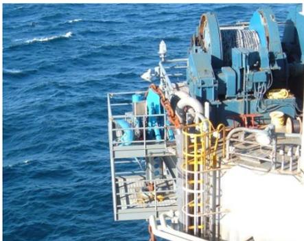
Bardex has designed and supplied supplemental mooring systems for floating drilling and production platforms to increase the platform's total mooring integrity and capacity so that the MODU or production vessel can stay on station and ride out a storm or hurricane rather than having to interrupt operations and run before the storm to seek shelter.
