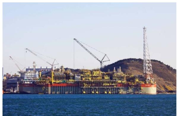
CLOV is an acronym for the names of the four fields - Cravo, Lirio, Orquidea and Violeta – found in the Angola Block 17 that the FPSO will produce from, with first oil expected in 2014. The FPSO is designed for a 160,000 bbls/day production capacity and will be moored in over 1,300 m water depth.
